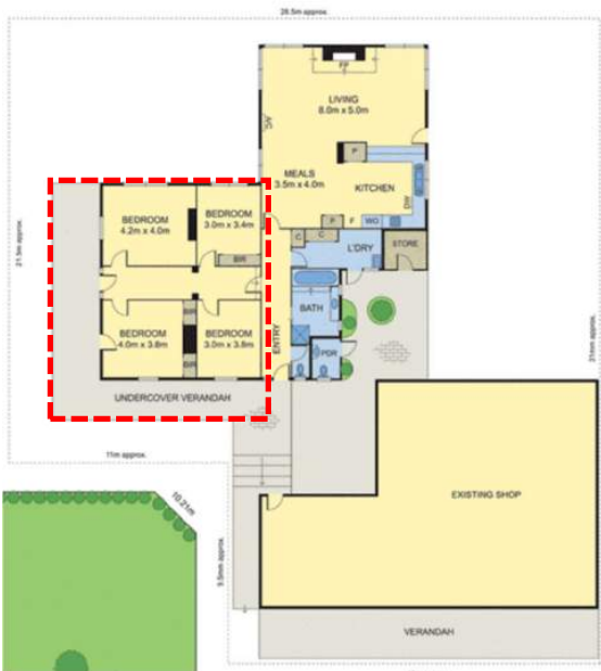
Figure 3: Floor plan showing the original four roomed house (indicated in red) with rear extension and shop. Source: realestate.com.au
