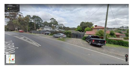
Figure 9: Example of existing roadside conditions at 413 Ryans Road Diamond Creek (Google Street View looking south, east on left hand side, west on right hand side), showing a constrained ability to provide a footpath on the western side of Ryans Road due to roadside parking
