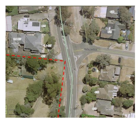
Figure 7: 405 Ryans Road Diamond Creek (red dotted line), showing DOT owned property projecting into road reservation, requiring a footpath on the western side of Ryans Road within the DOT owned property
